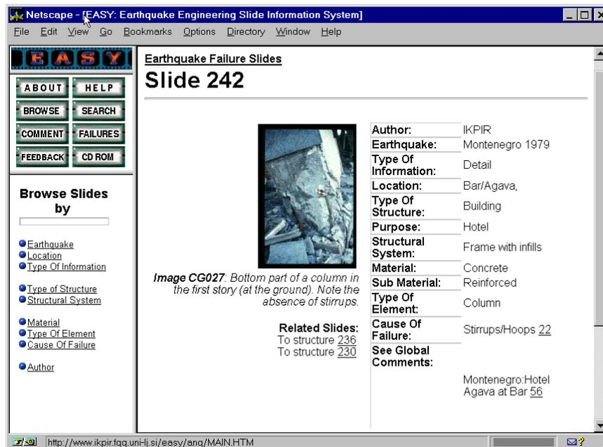
Figure 3 Detail of the structure on the Figure 2
